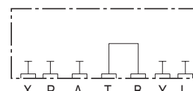
HXPC8TB* T to B-Port, P & A Blocked
