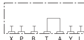
HXPC7TA* T to A-Port , P & B Blocked
