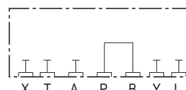
HXPC7PB* P to B-Port , T & A Blocked
