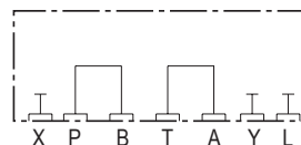
HXPC7PBTA* P to B-Port & T to A-Port
